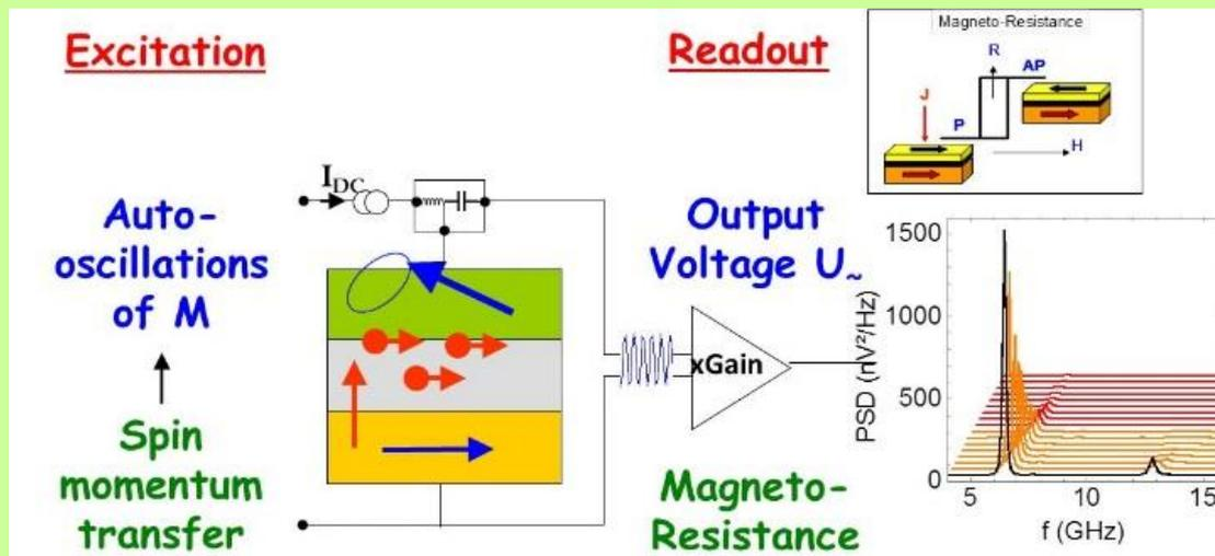
**Fig. 1:** Schematics of a spintronic microwave signal generator, showing to the left the spintronic heterostructure, into which a DC current is injected. Spin momentum transfer excites steady state magnetization oscillations that result in a microwave voltage signal due to the MR effect. The power spectra show the frequency shift of the microwave emission peak upon increasing current. The inset shows the MR effect.
