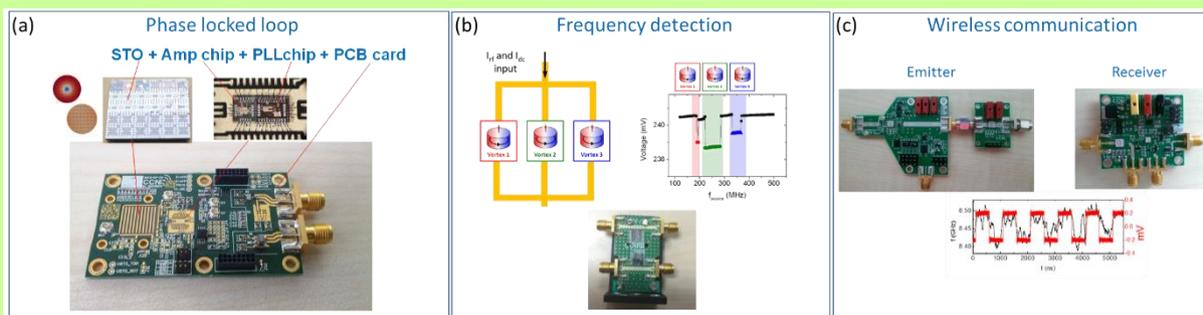
**Fig. 2:** Developed test systems: (a) PLL card including integrated PLL and amplifier chips, for homogeneous and vortex devices; (b) Example of simultaneous frequency detection using three different vortex STO devices, responding at different frequencies; (c) FSK based wireless communication with first test results for homogeneous devices.
